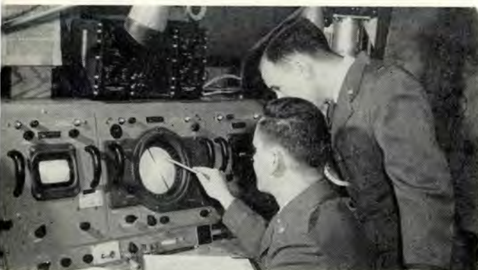
Locating dangerous storms up to 300 miles away and accurately measuring cloud heights, this AN/CPS-9 storm detector radar gives AWS important advance information on storms.
